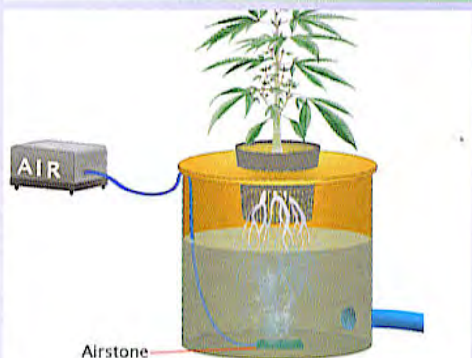
Cutaway of the inside of a DWC garden
