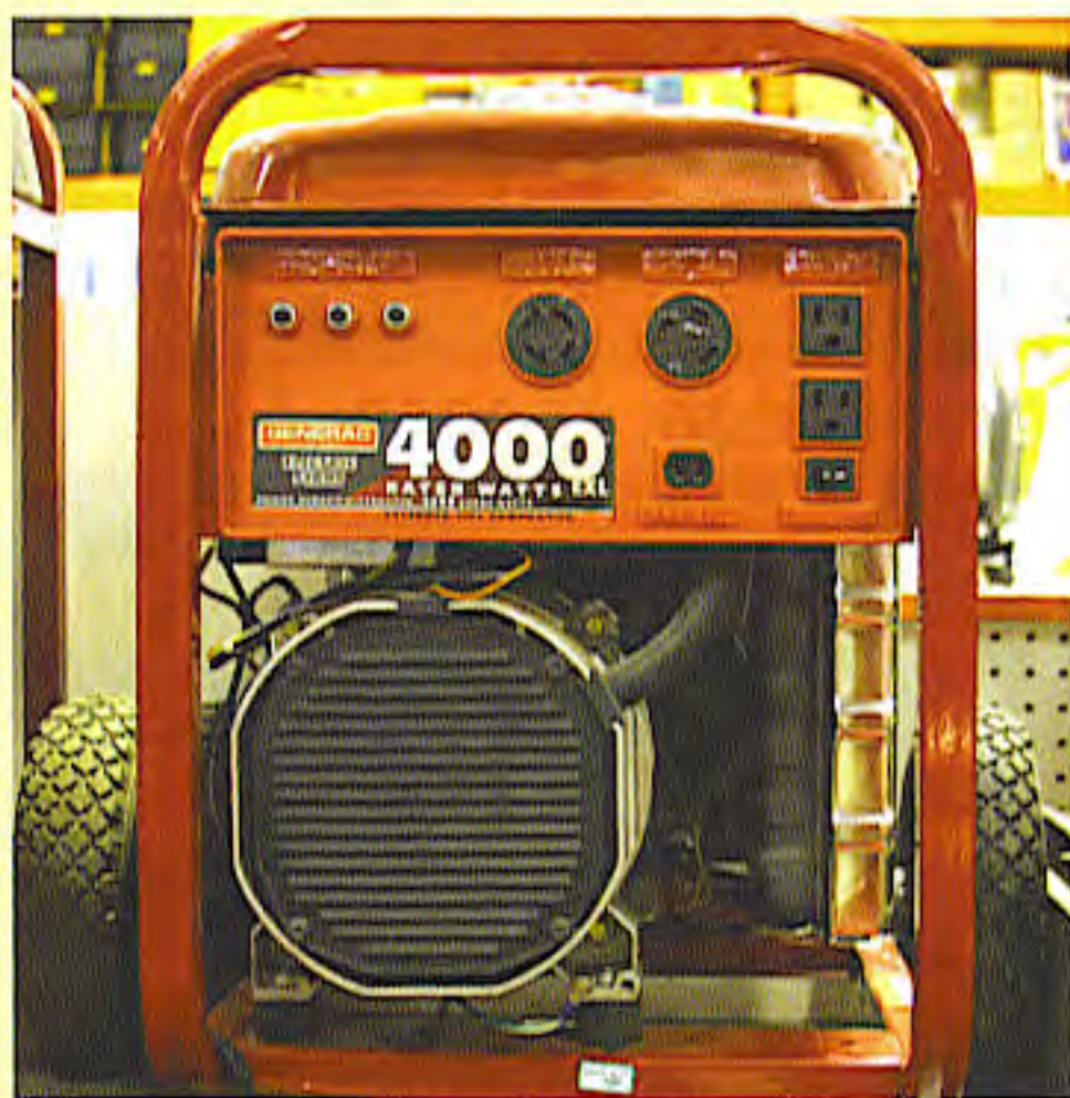
This generator produces 4000 watts at full capacity.
