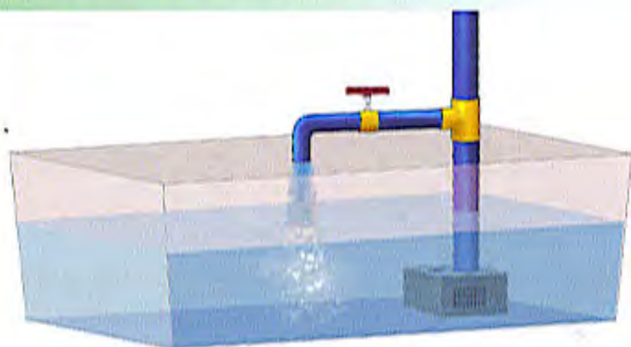
Attach a recirculating pipe with an on/off valve to the pump outlet pipe. This is a convenient and easy-to-control method of aerating the nutrient solution.
