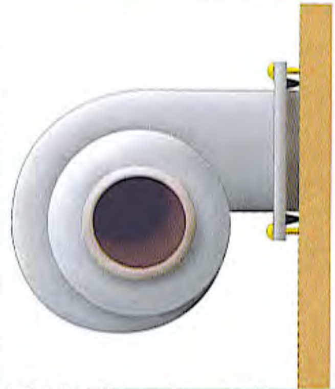
Put rubber feet on fans and blowers to shunt vibrations and noise.
