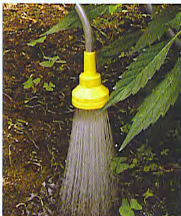
A water wand with an air breaker head oxygenates water and splits it into many streams.
